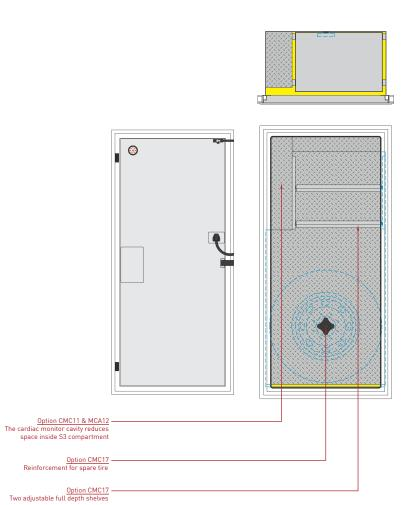
Option CMC11 & CMC17 Full height storage compartment [53] with two adjustable full depth shelves and reinforcement for spare tire Option MCA14 or MCA16
