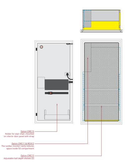
Option CMC11 & CMC15 Full height storage compartment [53] with two adjustable half depth shelves and stair chair holder on door Option MCA14 or MCA16
