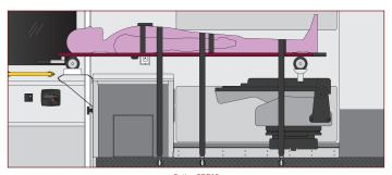
$\frac{\text{Option CDB12}}{\text{The 2nd patient mounted on FW \#107-C is installed and secured with foldable support on cabinet, removable support on rear wall and straps}$
