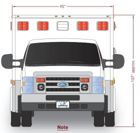
The total height of the vehicle can be different according to chassis and suspensions
