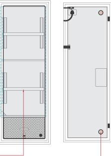
Option FBB12 ALS compartment with in/out access, two ajustable shelves, one fixed shelf and LED lighting
