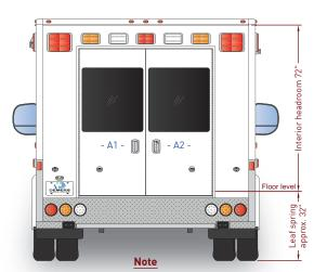
The rear loading height of the vehicle can be different according to chassis and suspensions
